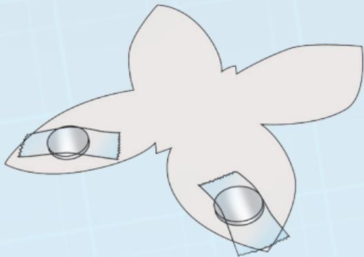
2. Because of the coins you taped on, the center of the butterfly's gravity is right at the head, rather than in the center. An object can be balanced if it is supported by its **center of gravity**. That's how you can balance it on your finger with your finger at its head.
