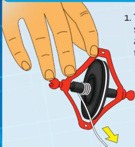
1. Thread the string through the small hole in the gyroscope's axis. Roll up the string around the axis.
